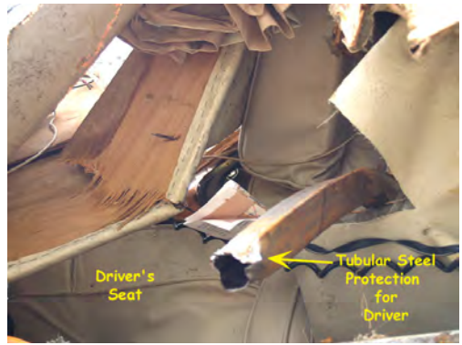
This 'sheetmetal' rollbar allowed the driver to be crushed.
