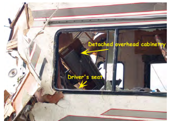
Driver was killed by a detached cabinet!
