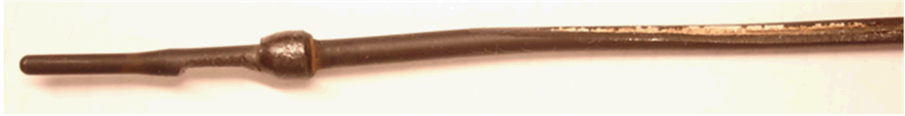
Figure 16. Damaged Thermocouple - Bent
