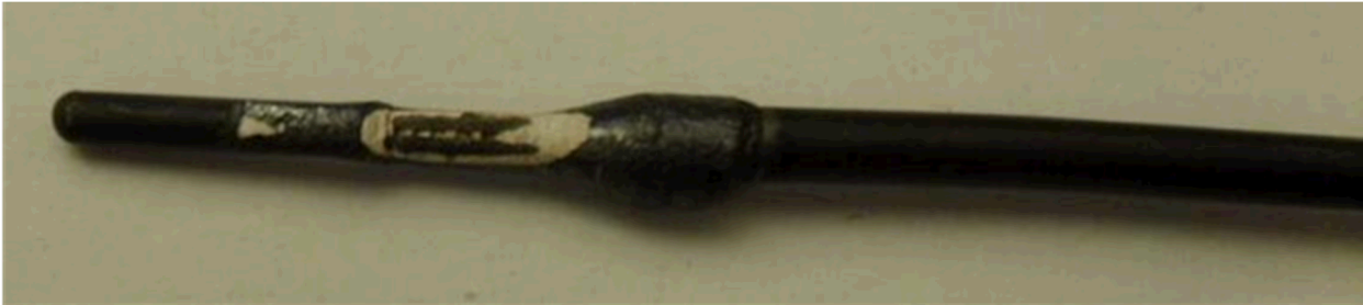
Figure 17. Damaged Thermocouple - Improperly Installed
