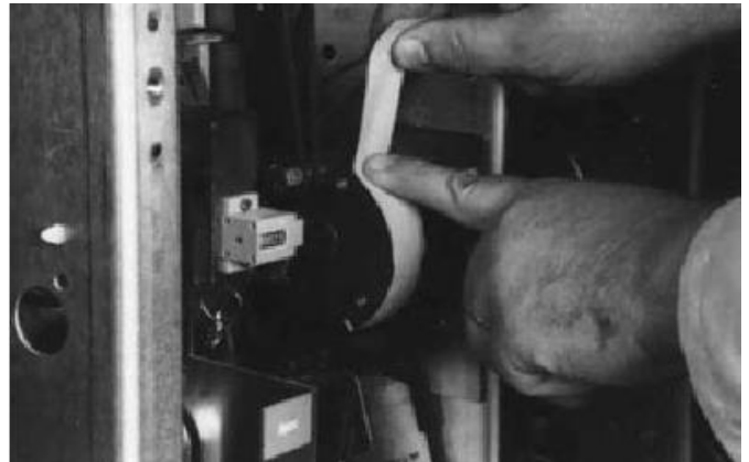
Figure 6-7 Wrapping Tape Up Around Cam
