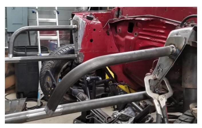
Once fitted appropriately, tack weld each tower plate to the shock tower as shown in the pictures below.
