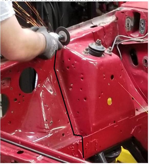
• Once the cut-lines have been marked, begin the cut at the top of the sub-frame with the cut-off wheel, making a 2-3" long cut on the inside face. This will allow the reciprocating
