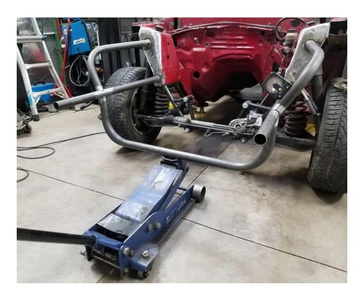
• Tack both ends of the radiator bar in place, on the inside and outside of the notch.
