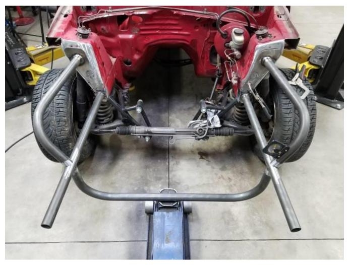
• At this point it's good to temporarily hang the fenders to check the alignment before final welding of the assembly.
