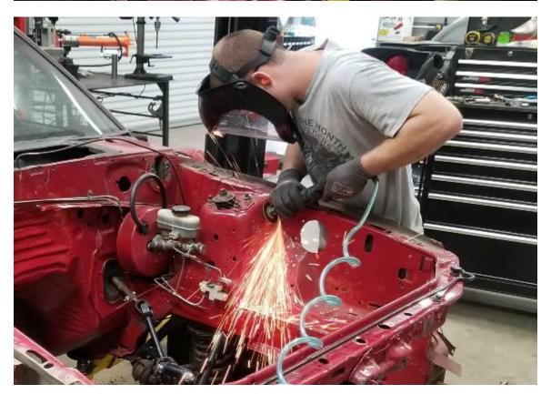
Cut the rest with the reciprocating saw; as shown below, it is recommended to cut the boxed frame square to the formed 'rail', and the upper fender boxed-section square to
