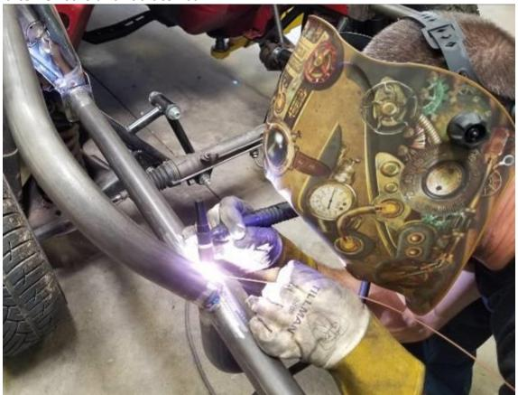
• Finally, fill in the gap left between the shock tower box and the frame tube mounting plate on both sides.
