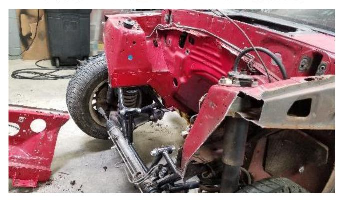
• Once the front sub-frame has been cut off, sand, deburr and clean the cut sheet metal edges. This will also allow you to even up any irregularities in the cut and remove sharp corners made from the manufacturing process where the sheet metal has been joined.
