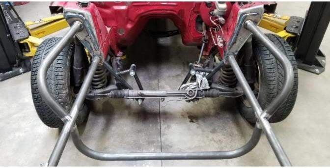
• Weld tower bars and radiator bar.
