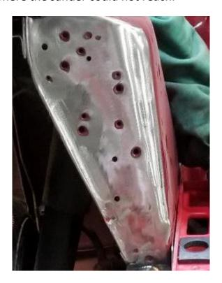
Pro-Tip: to aid in positioning the front frame-bars to the formed frame, we cut back the outer vertical portion of the frame rail "U" shape (inside shown) to allow the frame bar plate to rest in place. (This car previously had motor mounts added and removed, leaving a nearly rusted-through frame section which we had to repair.)
