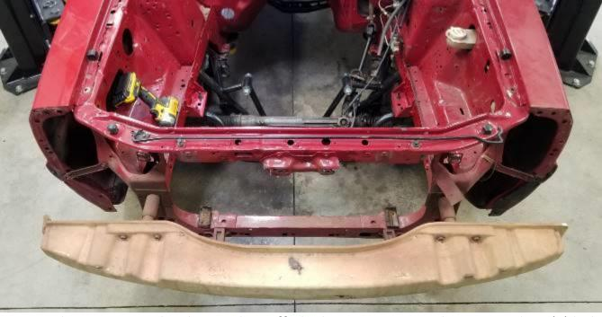
Once bumper cover has been taken off, the bumper core can be removed via (8) bolts.
