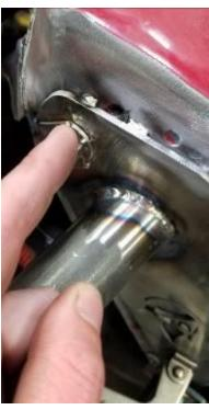
• Weld perimeter of tower plates. For the installation shown we welded in a counterclockwise path on the passenger side, and clockwise on the driver side.
