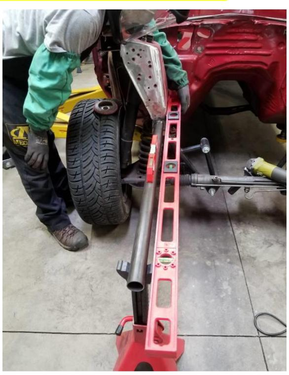
To match the frame bar elevation angle to the chassis, use a level or angle-finder to
