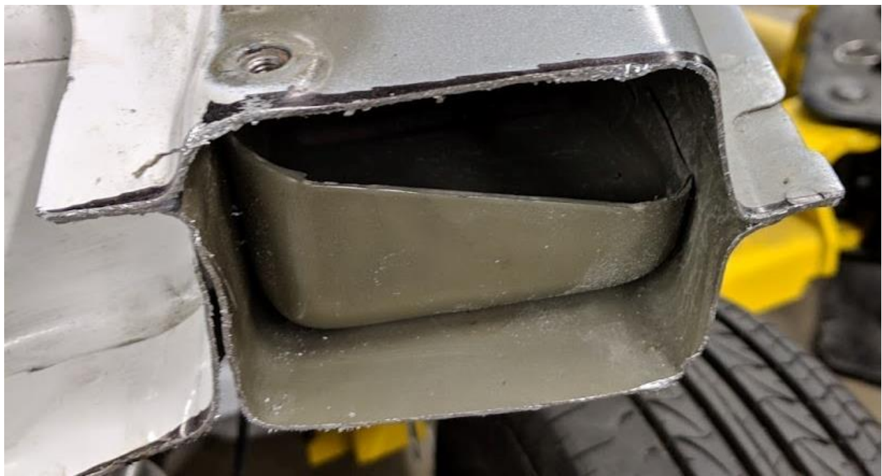
(End view of cut fender structure – note the formed metal brace on the interior)
