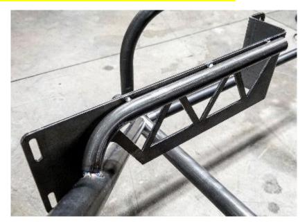
• Below are pictures showing the OEM headlight brackets attached to the RSM brackets:
