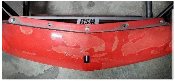
C. Remove the bumper cover and fully weld the bumper plate support tubes.
