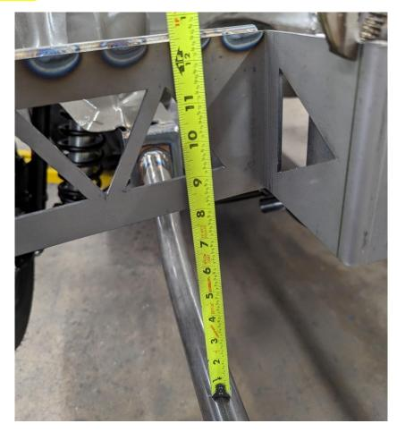
E. Front-to-rear = <u>Your measurement taken before teardown</u> – or approx. 12-3/4" from the face of strut tower to the front face of the long leg of headlight bracket. (~15-1/2" from the sheet metal seam on top of the strut box – see pic below)
