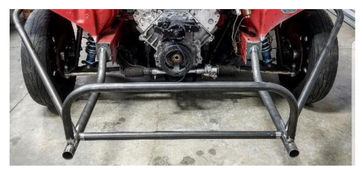
B. At this point you can go back and fully weld the kit. If you know where the cross tube needs to be final located, weld it in as well.
