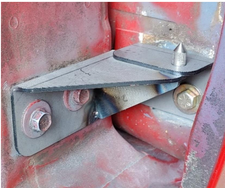
DRIVER SIDE LOWER HINGE INSTALLED
