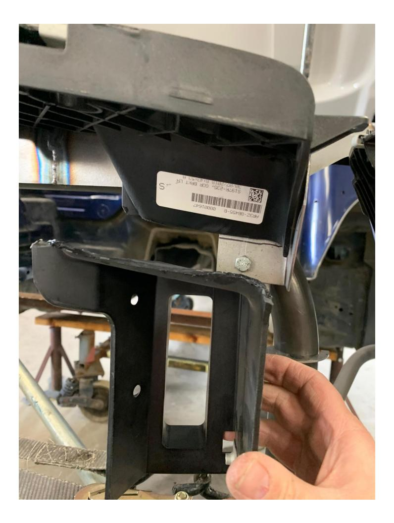
3. Fit and mount fascia; once in place drill holes for brackets into plastic support and mid-brackets on tube front.
