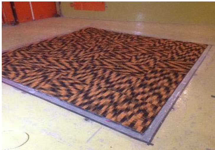
Figure 2: Carpet tile installed in chamber and ready for testing
