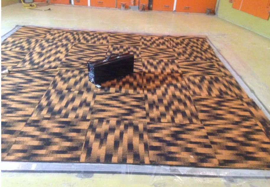
Figure 1: Sample installed in chamber with tapping machine on sample.
