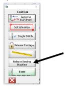
The following message will show on your screen letting you know QCT5 is no longer controlling the machine, allowing you manual control of the machine. *After* sewing test stitches off to side and making any needed tension adjustments, touch "**OK**" on screen message to return control of the machine back to QCT5.
