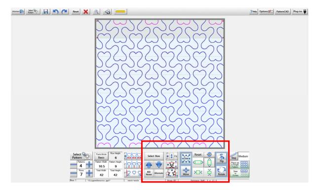
If I use a pattern that is already designed to be interlocked I can end up with spaces at the top and bottom of the quilt that don't have any design in them. By taping the Horizontal and Vertical clipping icons (shown below the Fit icon), I can change how the design looks.
