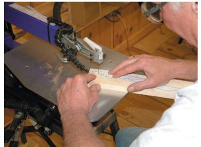
just start at the upper section of the mouth and continue cutting (photo 3.10) past where the fin is (was) and onto the belly on the back side of the fin and continue along the belly and then off the end of the part. Remember that this belly section and the dark section have to match up so saw slowly and put the middle of the line on at the middle of the blade and remove the entire line. Now you can start sawing at either end
