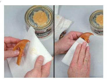
parts before they need to be changed. When it's time to change the towels, the "buffing" towel can be used to wipe off the excess and then a new towel would be used for the "buffing" towel. I will coat two or three pieces before I start to wipe the parts off, I wipe all of the parts and then start the process all over again until all the parts have been coated. We allow the first coat to dry over night to make sure it has dried thoroughly. The second coat can be applied the same way
