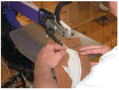
cut and proceed toward the tail where the point is. Once you reach the point in the tail, back out of the cut and reverse the direction and cut toward the head, do not follow around the dorsal fin but just continue cutting along the back (we will get to the dorsal fin later) and around the head and then finally off the part. Next, enter the part at the mouth area and continue cutting until you reach the fin, and go past the front part of the fin and then follow the fin on it's back
