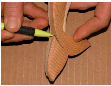
with the tail, remove the tail flipper. Smooth the tail along the top edges.
