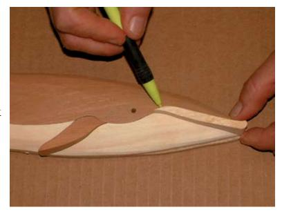
**Step 5.** Next put the white lip section back in place and mark around it with your pencil. Make this section just slightly thicker than the parts around it (about 1/16" thicker). Watch your pencil lines. If you do happen to sand below the lines, just lower the parts around it and start over again.
