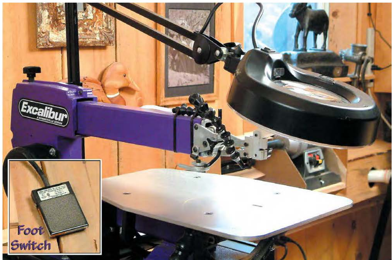
PHOTO 1.9 A foot switch and a magnifier with a light are great assets for scroll sawing.
