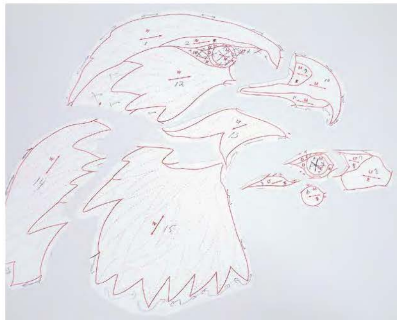
PHOTO 1.6 Cut the different sections, leaving a ¼" (6mm) border around the line work. Transfer the numbers from the master copy to the parts and mark the outside edges, as we have done with arrows.
