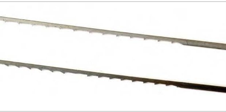
PHOTO 1.8 Plain-end blades are available in a variety of sizes. Reverse-tooth plain-end blades, shown here, usually give a cleaner finish on the bottom side of the part.
