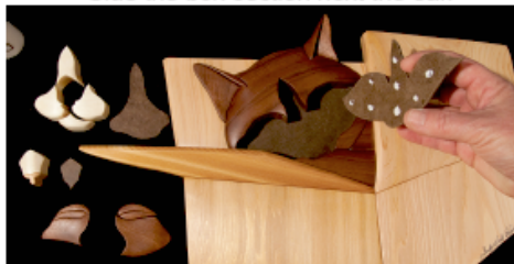
Glue the shims after adjoining parts are glued.
