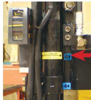
Correct fork height for entry and exit of pallet By matching the indicator sticker with the color marker, the correct fork height is obtained to enter the pallet safety.
