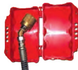
Forklift Propane Connectors
