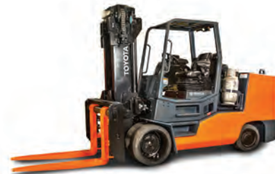
THDC Sit Down Cushion 18,000 - 110,000 lb. lifting capacity
