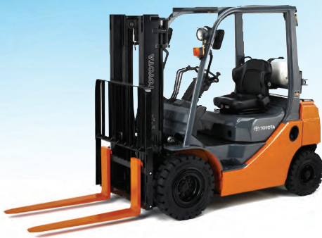
8FGU/8FDU Series • 3,000 - 6,500 lbs. capacity
