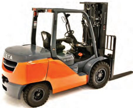
8FGU/8FDU Large Capacity • 13,500 - 17,500 lbs. capacity
