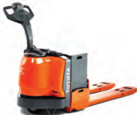
8HBW Electric Pallet Truck • 6,000 and 8,000 lbs. capacity
