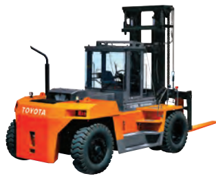
THD Sit Down Pneumatic 15,000 to 250,000 lb. lifting capacity
