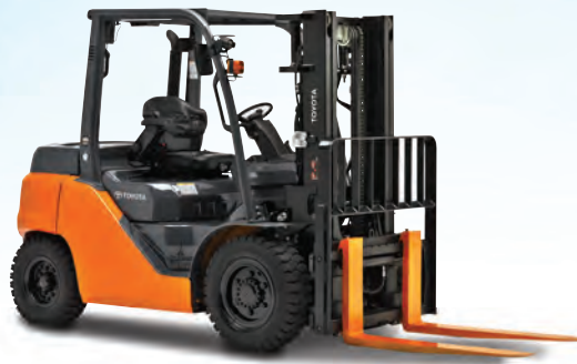
8FGU/8FDU Series • 8,000 - 11,000 lbs. capacity
