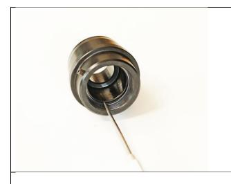
Step 4 – Using a pick, find the end of the Spiral Lock and stick the pick under it to remove the Spiral Lock from the body. Clean any grease or dirt off and set aside, you will need this to rebuild.
