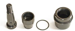
Step 5 – Remove the Internal Race from the Ball Joint Housing and set aside. All the pieces should now be out of the housing. Clean the housing of any grease, dirt and debris as best as you can.
