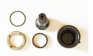
Step 4 – Remove the Top Race and the pin from the housing and set aside. You do not need this any more if you have a new rebuild kit as it will contain 2 new races and a new pin.
