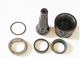
Step 5 – Remove the Bottom Race from the Ball Joint Housing and set aside. You will not need this race any longer if you have a rebuild kit. All the pieces should now be out of the housing. Clean the housing of any grease, dirt and debris as best as you can.
