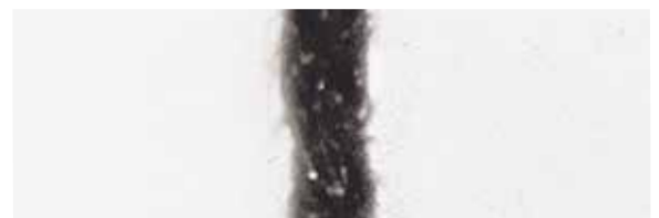
Ring spun yarn provides higher strength to fabric
