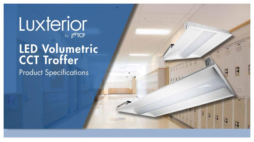
TCP's LED Volumetric CCT Troffers offer a high-efficiency alternative to T5, T8 and T12 linear fluorescent systems. They provide long life with consistent color and superior lumen maintenance. Designed to mount in a variety of grid ceilings, the rugged, cold-rolled steel housing is post-painted with a highly diffuse white finish. The low-glare acrylic diffuser provides wide distribution and the sloped reflector softens the contrast between the luminaire and ceiling.
