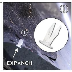
**FIGURE J** Logo-side of flap facing vehicle rear, position against liner mounting points. Install SMWASH & 1SS#8 into mount 1 through flap and EXPANCH.
