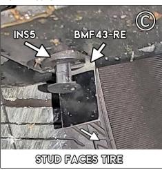
**FIGURE D/E** Install SMWASH with SSLNUT onto mount 1, stud of BMF43-RE. For mount 2, align upper flap section against fender flare then position RACLP onto flare and flap. **Fully install RACLP after confirming flap is parallel to even ground**. **FIGURE F** Fully aligned, install RACLP to mounts 3 & 4.
