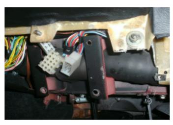
10. Remove the original mounting brackets LH/RH
