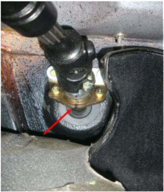
3. Allign the steering system to their neutral position and mark the steering shaft to the firewall.
