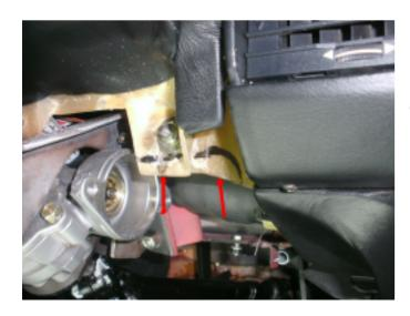
12. In some cases it's necessary to remove a small piece from the dash. See photo for cutting line, which is drawned with a marker.
