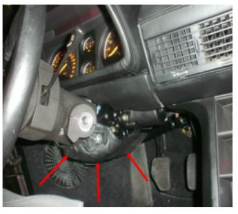
21. Nicely fit all wires underneath the dash. Refit the leather dash cover.
