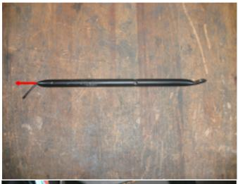
15. Bend the long end from the RH mounting bar to a straight position and fit the bar to the unit.
