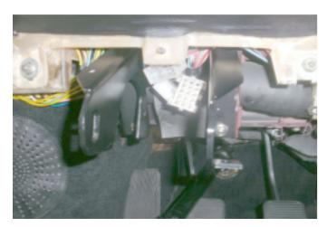
9. Disconnect the connectors and remove lower mounting bolts. Remove column afterwards.
