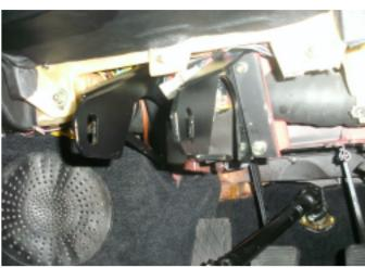
14. Fit the mounting brackets from the powersteering kit.
