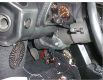
4. Remove the leather protection from the steering column.
