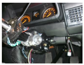
16. Fit the steering column switches to the powersteering unit.
