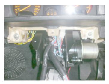
14. Fit the universal joint from the steering shaft to the unit and fit the lower mounting bolts. Let the unit pivot at the lower bolts to get acces to the connectors. Reconnect them and raise the unit to the right position to fit the height adjustment bolt.
