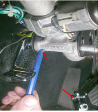
7. Remove tension pin from the height adjustment from the original steering column.
