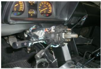
6. Remove steering column covers to get acces to the steering column switches. Remove these switches.
