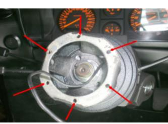
5. Remove the steering wheel, Remove the small outer bolts first to get acces to the central mounting bolt.
