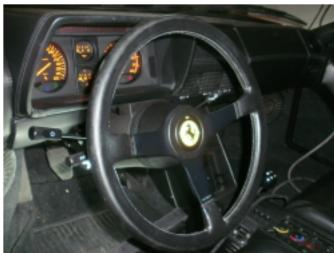
17. Fit the steering column covers and the steering wheel.
