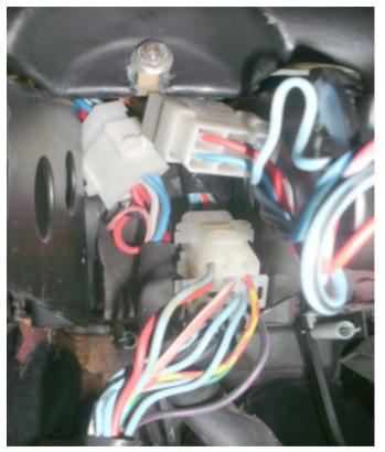
8. Remove height adjustment pin and let the column pivot at the lower mounting points to get acces to the connectors.
