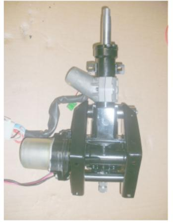
11. Remove the original ignition lock from the original steering column and fit this to the powersteering column.
