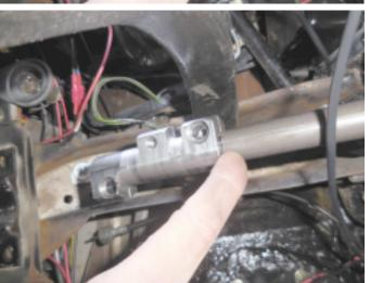
14. Install both bolts and tighten them with 35NM / 26 FOOT/POUND. Do not forget the washers underneath these bolts!
