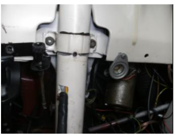
6. Remove the upper installation bolts from the steering column.
