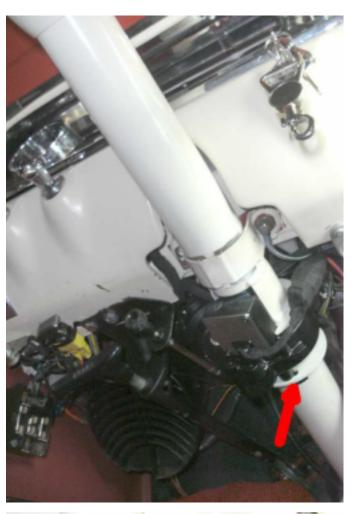
15. Install the EZ unit into the car en tighten it. The bolt from the clamp/adapter can be thightened through an opening in the output tube.
