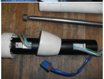
Do not forget to slide the lower part over the EZ column prior to the installation from the switch and wiring.
