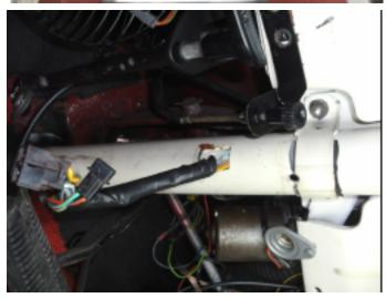
5. Disconnect the connectors from the steering column.
