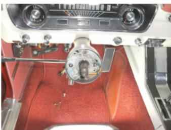
4. Unscrew the lever from the indicator switch.
