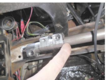
13. Clean/decrease the shaft after drilling and check if the clamp can be fitted over the original steering shaft, see if the recesses are located OK to install the bolts. If all OK continue with the conversion.
