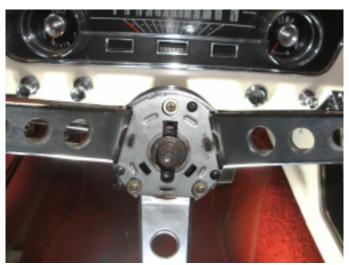
3. Remove the horn button and the steering wheel.
