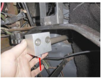
11. Slide the drilling tool over the remaining original steering shaft. Lock the tool with the bolt (red arrow). Now you can use the supplied 8.5mm drill to drill the recesses in the steering shaft.
