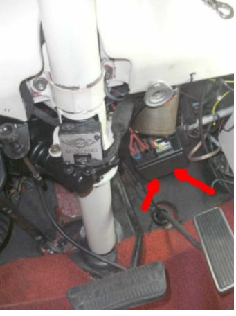
16. Locate a suitable location for the EZ ECU and install it. Connect the EZ wire harness with the ECU afterwards.
