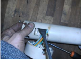
8. Remove the indicator switch from the original column en install in onto the EZ unit.
