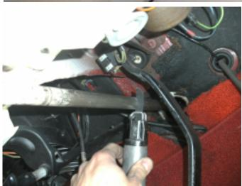
10. Measure this distance back from the top of the orignal steering shaft. Mark this and cut the shaft. Be sure that there will be a straight cut.
