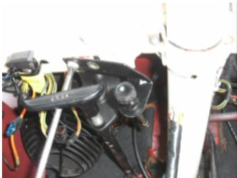
7. Remove the installation bolts from the parkbrake bracket.
