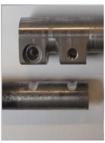
12. These recesses are needed to give enough clearance for the clamping bolts from the clamp.
