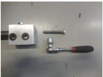
11a. To remove the drilling tool from the shaft, there is thread tapped at the back of the tool, Use a long M8 bolt to push the tool of the shaft.
