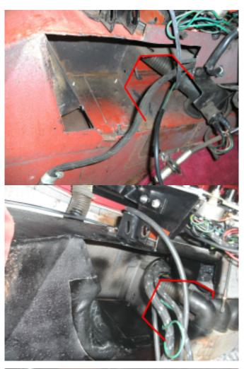
9. For the second cut, again use the foto to determine where to cut and cut out the excessive material.
