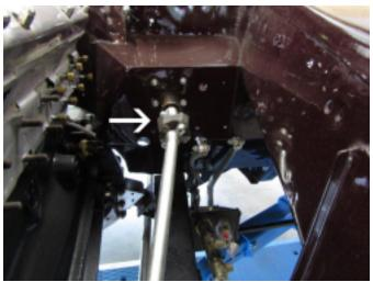
6. Remove the installation bolt from the steering shaft coupling in the engine compartment.
