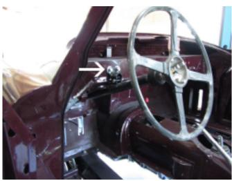
7. Remove the upper installation bolt from the column and remove the complete column from the car.
