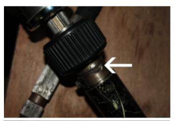
4. Remove the 3 allen bolts to remove the hornbutton, also disconnect the horn wire. Remove the indicator switch with cover. The indicator reset can be removed also.
