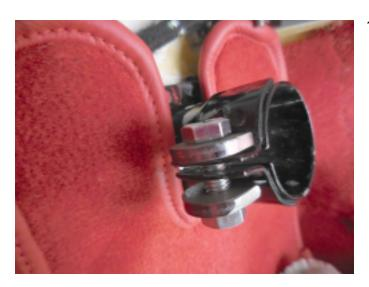
11. Install the washers with bolt (8x25) at the clamp at the firewall.
