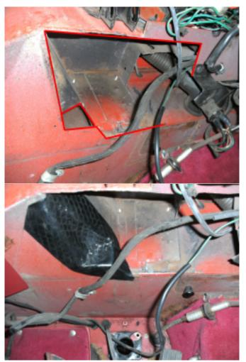
8. To get enough clearance for the EZ unit some excessive material underneath the dashboard needs to be removed. When the EZ unit is installed the servo motor can be placed in there.
