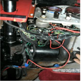
10. Install the EZ unit, slide the output shaft into the steering shaft coupling, then install the upper installation bolt, do not fully tighten it yet!
