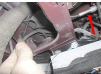
10. Mount the speed sensor between the speedometer and cable.
