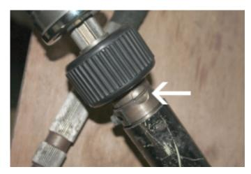
3. Remove the retaining grubscrew from the steering shaft. Subsequently the steering wheel can be removed. Please note, the horn wire must be cut!
