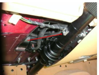
14. Connect the original horn wire to the spring contact at the side of the EZ unit.
