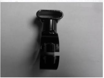
11b. See photo, at an XK140 OTS the upper mounting point is relocated compared to an coupe version. An adapter is supplied to solve this. Slide this over the EZ unit, use the original column for the right location.
