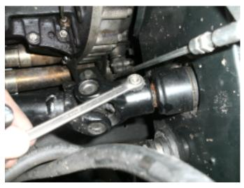
4. Remove the nut from the taper pin of the universal joint. Use a hammer with a drift to remove the pin itself.
