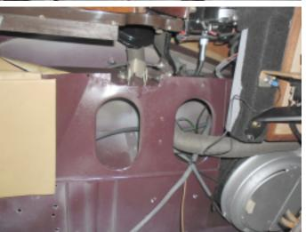
7. To gain space for the EZ unit, it is necessary to remove excessive material. Use the template, to decide where to cut. NOTE: this manual is for a LHD car, normally a RHD car is the mirror image from a LHD. In case from a RHD, double check with the EZ unit to decide were to cut.
