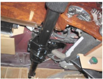
12. Mount the EZ unit in the car. The mounting points from the EZ unit are fitted with clamp bolts. As a result, it is possible to turn the column in the right position. Do not forget to fasten the clamps again together with the remaining mounting bolts!
