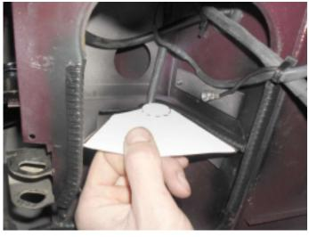
9. Use the template to cut the last piece of excessive material. It is recommended to paint the cut edges and then fit rubber edging over sides of the metal.
