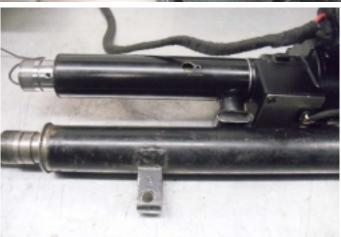
11a. Compare the original steering column with the EZ unit. A difference in length can be be up to 17.5mm, this is within original Jaguar specs.
