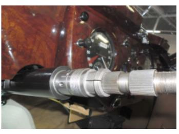
Mount the steering wheel and connect the horn-switch with the horn wire of the EZ unit. Subsequently, mount the horn switch.
