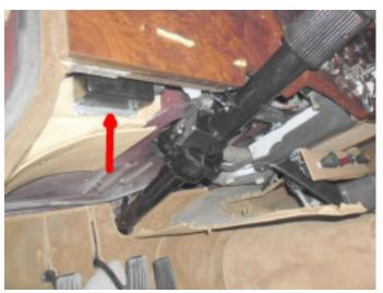
15. Find an appropriate place for the ECU and connect the wiring loom to the ECU.
