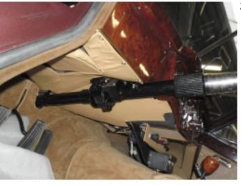
23. Install the cover under the dashboard and adjust if necessary.
