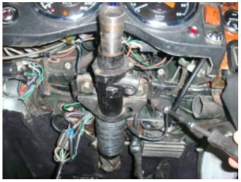
9. Remove the 4 mounting bolts from the upper mounting bracket underneath the dash.
