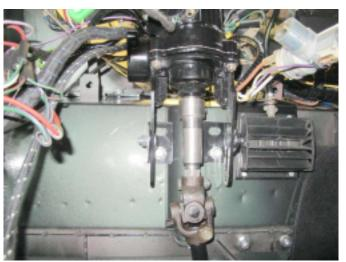
11. Remove the electric motor from the EZ unit and install the unit in the car. Slide it into the u-joint first. Do not tighten the bolts yet.
