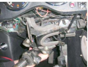
10.Remove complete steering colum with bracket from the car. The U-joint stays in the car.
