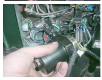
13. Install the electric motor back on the EZ unit.
