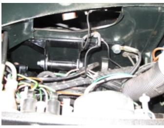
11a. De upper mounting bolts are reachable through the top now that the upper dash has been removed. When the column is located/aligned correctly, tighten ALL mounting bolts, included the U\_joint and output shaft
