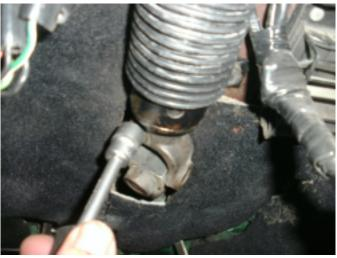
8. Remove mounting bolt from the lower U-joint.
