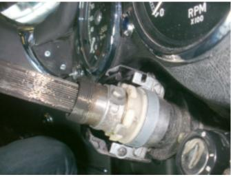
5. Remove indicator switch from the original steering column.
