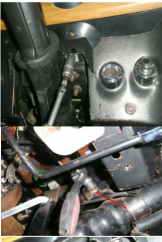
9. Remove column mounting bolts and remove the steering column from the car.
