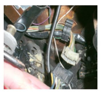
8. Disconnect connector from the indicator switch.
