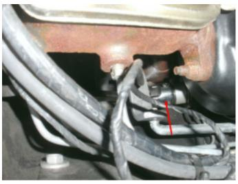
14. Connect the steering coupling in the engine compartment, watch the allignment!
