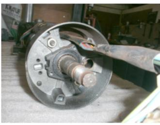
11. Remove tension ring with the 2 bolts Remove the top holder afterwards. This holder can be installed on the EZ column, together with the indicator switch.
