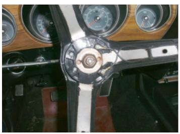
5. Remove steering wheel nut and remove steering wheel.
