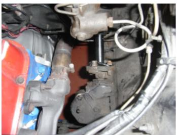
3. Disconnect the steering coupling in the engine compartment
