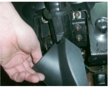
6. Remove steering column cover to get acces to the mounting bolts from the column.
