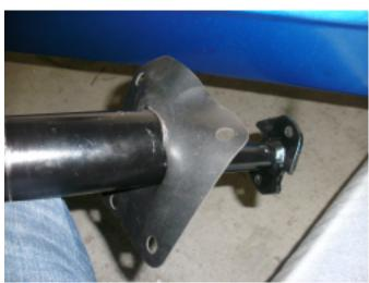
12. Install the original rubber seal onto the EZ column. Be sure that the EZ clamp already is installed on EZ unit.
