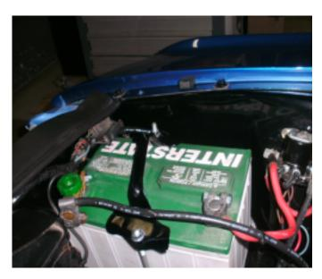
2. Disconnect the batterie earth and allign the steering system to its center position, mark this position.
