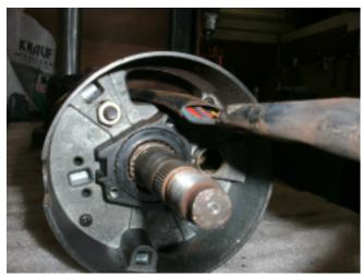
10. From the removed steering column the indicator switch must be removed.
