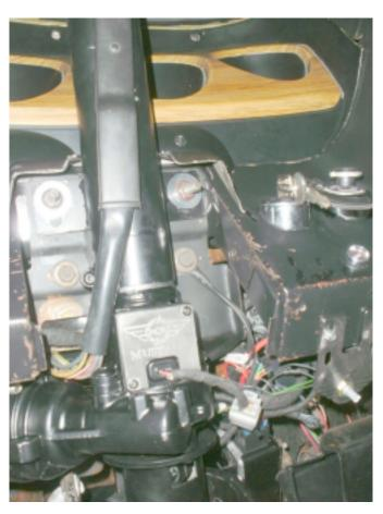
Install the EZ column in the car. The indicator switch connector can also be connected.
