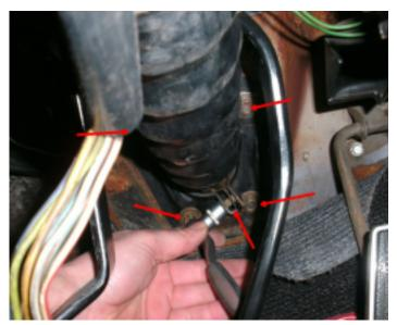
7. Remove mounting plate against the firewall.
