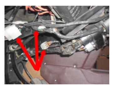
5. Disconnect the steering column connectors (steering column- and ignition switch).
