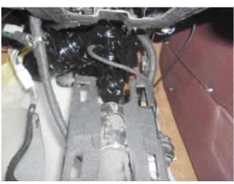
10. Connect the original U-joint from the upper column to the EZ unit.
