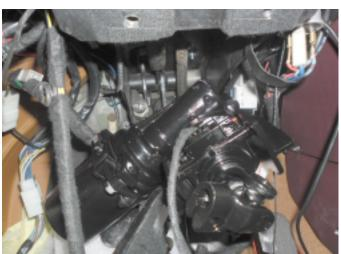
9. Install the EZ unit in the car and connect the output shaft/joint with the original steering shaft.
