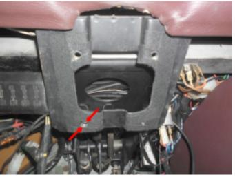
8. From the original fixing points there are 2 M6 threaded. One of them needs to drilled to 8.5mm. See photo.
