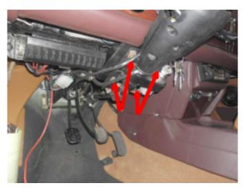
Remove the bolt which holds the Ujoint to the steering column. Remove the 4 mounting bolts from the upper column and remove it afterwards.
