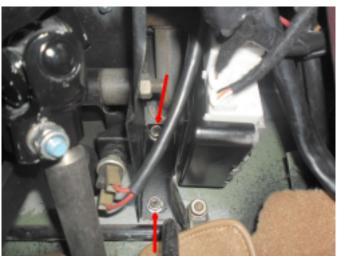
13. Install the EZ ECU with it's bracket against the firewall.
