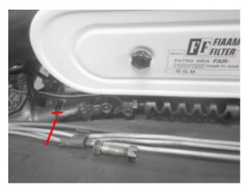
3. Mark this position on the steeringbox, also mark the position from the U-joints against each other.
