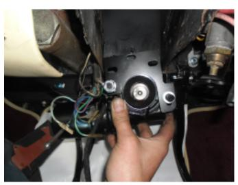
11. Install the EZ bracket onto the unit (do not tighten the bolts) and install the EZ unit. Also fit the outputshaft to the unit.
