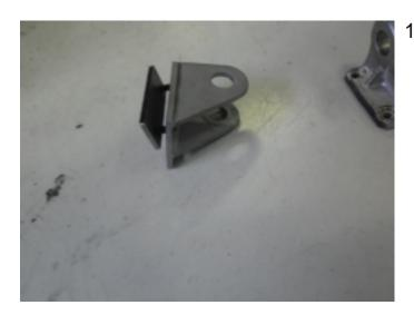
10. Temporarly install the throttle bracket, it's needed to drill 2 holes (6.5mm). Mark both holes and drill them after removal from the bracket. Remove pedal from original bracket and install it into the EZ one. Install the complete pedal assembly into the vehicle.
