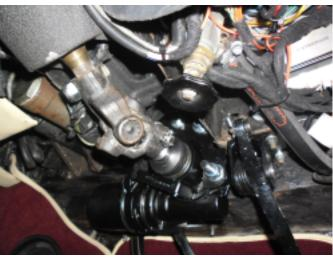
12. Reinstall the upper steering column into the vehicle, watch the alignments from the u-joints and steering box (see point 3). Reconnect the steering column connectors (see point 6). Be sure the EZ unit is aligned correctly and shafts are fitted tension free (axial and radial)! Tighten all nuts and bolts after this has been done.
