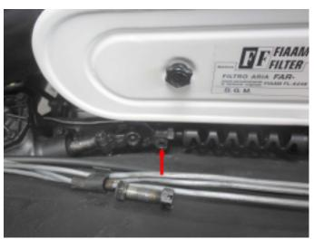
4. Remove bolt from U-joint at steering box.
