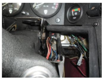
6. Remove bolt from U-joint underneath steering column. If needed remove cover at the top from column. Disconnect the connectors from the steeringcolumn. After removal from the mounting bolts the column can be removed from the car. The throttle pedal can be removed afterwards.
