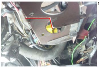
9. To give the powersteering unit enough clearance some material needs to be removed around it. See photo's and supplied template for this.
