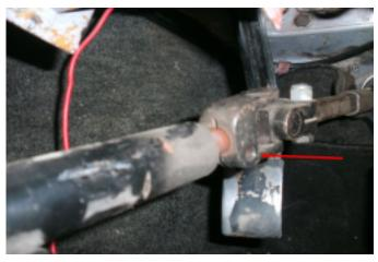
5. Remove mounting bolt from the lower u-joint.
