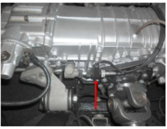
11. Fit he speedsignal adaptor between the speedometer cable and gearbox.
