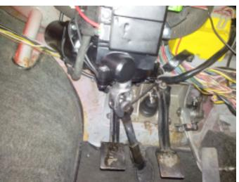
10. Slide de axle from the powersteering unit (with unit) into the original steering shaft. Watch the plastic guides. Mount the unit with bolts to secure it.
