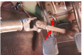
8. The original sliding shaft can be pulled out the original axle. Remove the plastic guides from the original axle and fit them to the new one.
