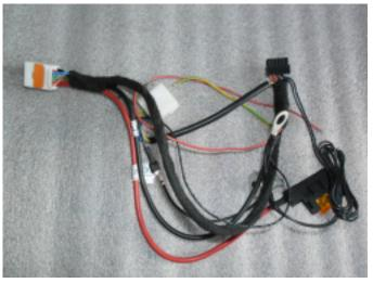
Connect the wire harness with the powersteering ECU.
