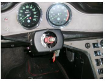
17. Fit the steering column switches with the covers at the steering column.
