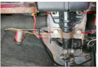
6. Remove the mounting bolts from the steering column.
