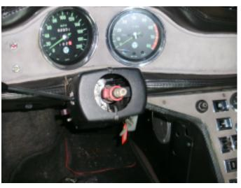
4. Remove covers and steering column switches.
