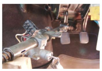
7. Steering column can now be taken out of the car. (take care with the ignition switch with wires!) Remove the ignition switch from the orginal steering column and fit it to he powersteering unit.
