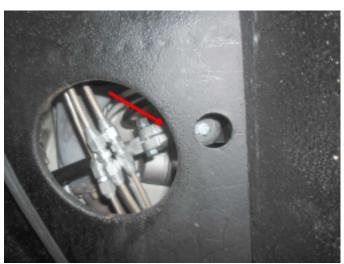
6a. If needed remove the cover in the inner wheel arche to get acces to the U-joint.
