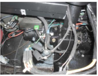
17. Install the upper part with switch back onto the EZ unit. Reconnect the connectors from the steering column switch.
