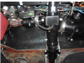
18. Fasten all wiring underneath the dashboard and install the cover underneath the dashboard.
