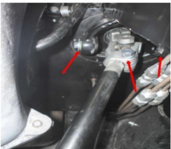
6b. Remove the bolt from the U-joint together with the lower mounting bolts from the original column.
