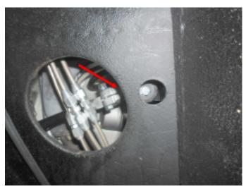
12. Install the EZ unit, slide the U-joint from the EZ unit onto the original steering shaft. (do not tighten the bolt yet).
