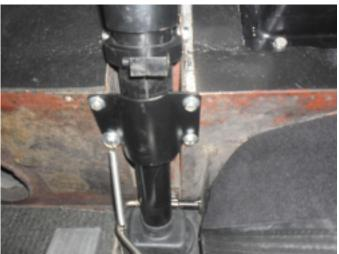
16. If available install the support bracket underneath the column.
