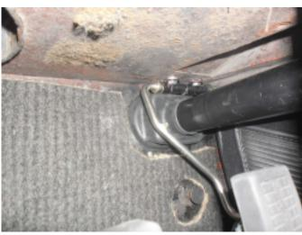
7. Remove the braid wire which holds the rubber gaiter at the firewall. Slide the gaiter up afterwards.
