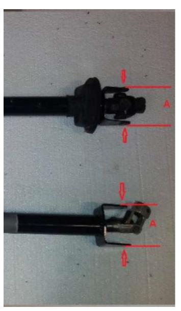
10. Before you proceed with the conversion, compare the width from the U shaped bracket from the original and EZ unit. They must be similar
