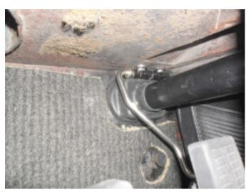
14. Install the rubber gaiter at the firewall and secure it with braid wire.
