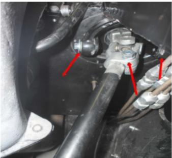
13. Now install the 2 lower bolts from the steering column.
