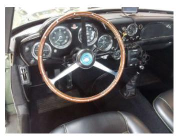
To remove the steering wheel, the bolt/nut which clamps the steering must be removed, also pay attention to the horn wire, when removing the steering wheel.
