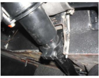
15. Install the upper bolt from the column, get the motor into the right position en tighten all bolts, do not forget the U-joint!!
