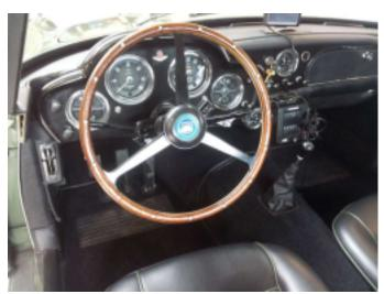
21. Install the steering wheel with hornbutton and take the vehicle for a testdrive and recheck all systems.
