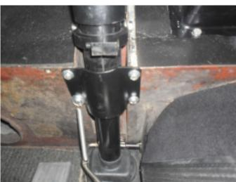
8a. If installed to the car, remove the support bracket underneath the dashboard.
