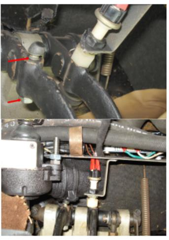
8. Once the bracket has been cut, the nut from the bolt on top of the clutch pedal needs to removed and fitted underneath the clutch pedal. Be sure to reset the position from the bolt to remain the same height from the clutch pedal afterwards. This bolt touches the EZ unit once it is fitted.
