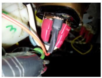
20. Connect the ignition switched positive lead (15+) to the ignition switch 15+. Check if this connection is switched on by the ignition first.
