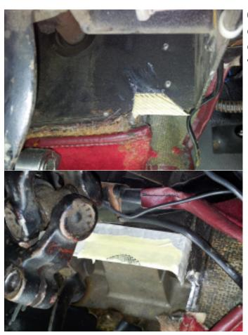
6. In the pedal box, material should be cut away for the EZ Powersteering electric motor. Use the template supplied with this manual.
