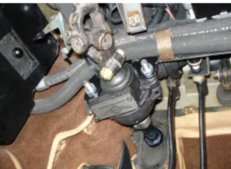
16. Tighten the bolts in the universal joint and in the steering wheel height adjuster. Use a new wire to secure the bolts on the universal joint at the steering box. Fit a new split pin on the bolt in the universal joint under the dashboard. Secure the aircon hoses with tie wraps to secure them so they cannot touch the u-joint.
