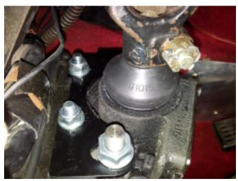
15. Fit 2 bolts (M8) from behind in the mounting bracket holes. Fit nuts with washers on the bolts' threads.
