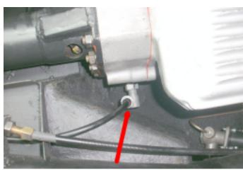
21. The speedometer signal is taken from a cable that runs from the transmission. Mount the adapter between the transmission and the speedometer cable. Use tie-wraps to run the lead along with the existing ones back to the car, and connect the lead to the EZ Powersteering computer.
