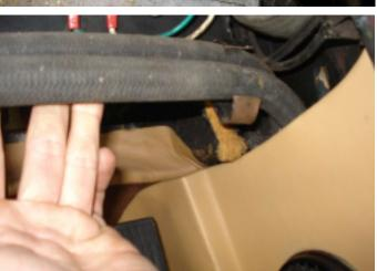
10. Loosen the clips which hold the aircon hoses. The hoses need to be rerouted slightly just above the unit. It would help if the aircon hoses are removed, there for the aircon system needs to be vacumed prior installation of the EZ unit and refilled after the EZ unit is installed. We advise you doing this. It's improves accessibility very much! But it's possible without.
