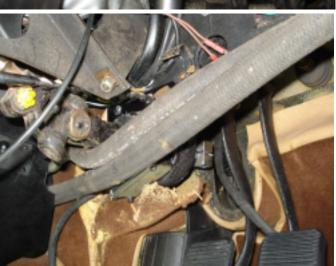
14. Check if the EZ unit turns freely and if there is enough clearance between the EZ unit and pedal box. If all OK, fit the nuts from the mounting bracket and adjust it into the correct position. Use a marker to mark the holes on the metal that is behind the mounting bracket, and drill these holes with a 9 mm drill. (if not removed, temporarly route the aircon hoses underneath the EZ Unit for accessibility.)
