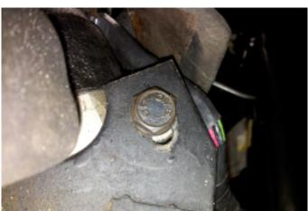
9. Slacken the 2 bolts in the steering column height adjuster. It can now move freely, making the installation of the electric motor easier.
