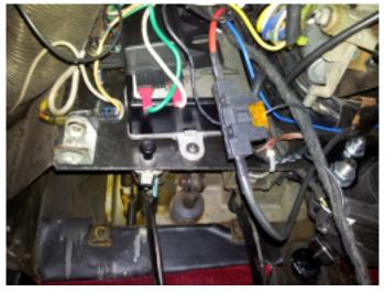
17. Mount the computer with its mounting bracket on the front of the pedal box.
