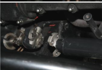
4. In the engine bay, release the steering shaft by cutting the securing wire and unscrewing 4 Allen bolts (4 mm). Use tape on the universal joint in the engine bay to prevent it from falling apart.
