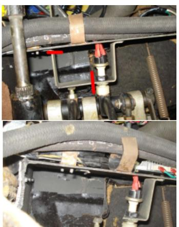
7. The Brake light switch bracket need to be modified. See photo, where to cut the bracket.
