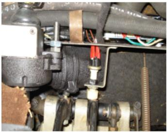
11. Install the electric motor by moving it upwards over the brake light switch first.
