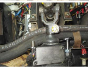
12. Slide the electric motor input shaft in the steering wheel side universal joint. Fit the bolt in the universal joint without tightening it. The aircon hoses are just routed over the universal joint (be sure they do not touch the U-joint), also fit the mounting bracket loosely into place. If not possible to fit both aircon hoses over the EZ unit, Then run the thickest hose underneath the EZ Unit.
