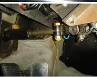
5. Unscrew the bolt in the universal joint under the dashboard. Remove the split pin. Remove the steering shaft. The rubber sleeve/grommet should be refitted in the bulkhead. Fit the EZ output shaft afterwards.
