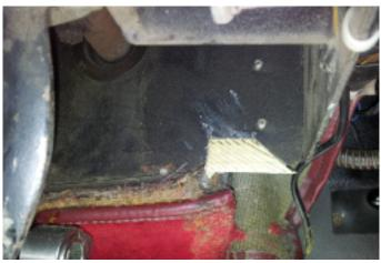
6. In the pedal box, extra room should be cut away for the EZ Powersteering electric motor. Use the template supplied with this manual. Tighten the bolts in the universal joint in the engine bay.
