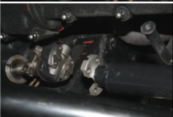
4. In the engine bay, release the steering tube by cutting the securing wire and unscrewing 4 Allen bolts (4 mm). Use tape on the universal joint in the engine bay to prevent it from falling apart.
