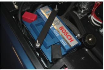
2. Remove the battery negative lead. Place the front wheels in a straight position.
