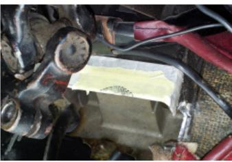
7. Slacken the 2 bolts in the steering column height adjuster. It can now move freely, making the installation of the electric motor easier.
