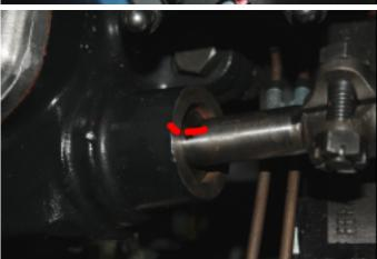
3. Mark the straight ahead position on the steering box. Also watch the allignment from the universal joints, they should be lined up. Sometimes they are not lined up OK, prior the conversion. Be sure to check/correct this.
