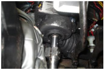
11. Slide the output shaft over the electric motor's splines.
