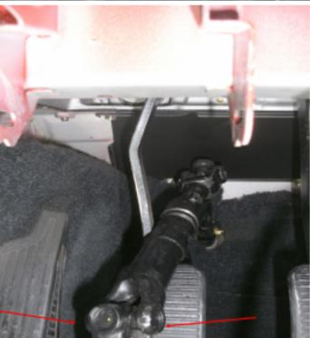
5. Remove the universal joint at the bottomm of the steering column. Remove the mounting bolts from the steering column and remove the steering column.
