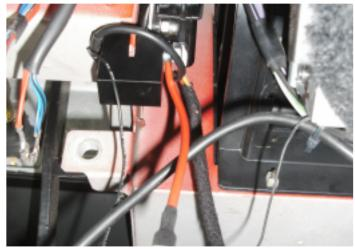
10. The ECU can be fitted just above the pedals, with the clamp/bracket
