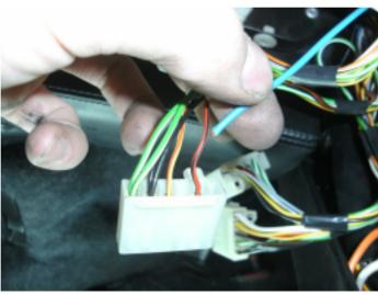
11. Connect the speed signal wire from the powersteering unit to the red/black wire from the speedo from the car. This can be located behind the removed instrument cluster. After the wire has been connected the instrument cluster can be refitted.
