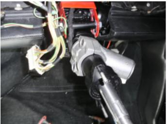
7. Remove ignition lock from orginal column and fit it to the powersteering column
