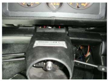
3. Allign the steering system. Mark this position on the lower universal joint at the firewall. Remove the steering wheel afterwards.
