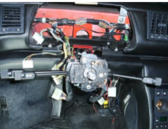
4. Remove the steering column cover together with the instrument cluster and the steering column switches. Watch the connectors!
