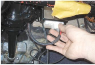
16. Connect the EZ wiring loom to the ECU.
