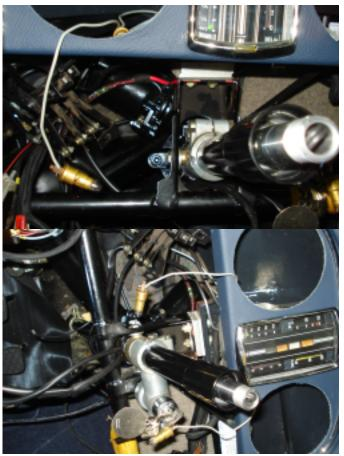
13. Mount the input tube on the EZ unit, together with the mounting clamps and where fitted optionally, the steering lock. Do not fasten the mounting clamps yet! In case the EZ unit has multiple contact pins on behalf of the indicator switch and horn, mount the contact pin holder after the input tube is stalled. Check the alignment in respect to the copper slip rings.
