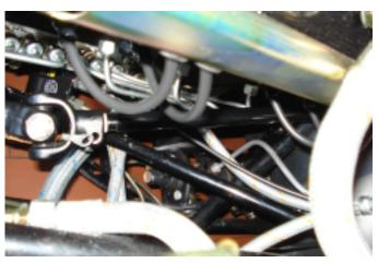
5. Remove the retaining bolt from the universal joint in the engine compartment.
