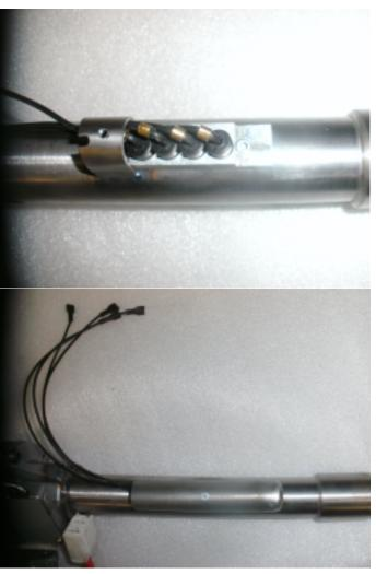
23. In case there are 4 contact pins it is necessary to fit the supplied cover under the steering tube over the contact pins between the dashboard and the steering wheel. This is tightened with an allen key.
