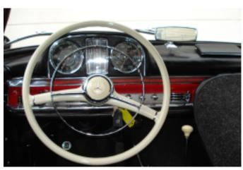
24. Mount the steering wheel. Connect the horn wire and optionally the indicator wires to the switch. Fix the switch in the hub of the steering wheel.
