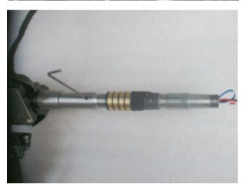
12. Install the input shaft on the EZ unit. Use Loctite to securely lock the M6 retaining bolt.
