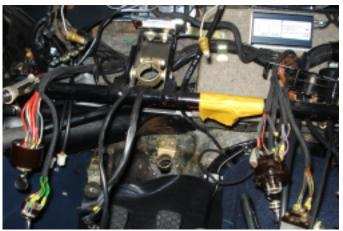
6. Once the mounting clamps of the original steering column have been loosened, the original steering tube and —shaft can be removed.
