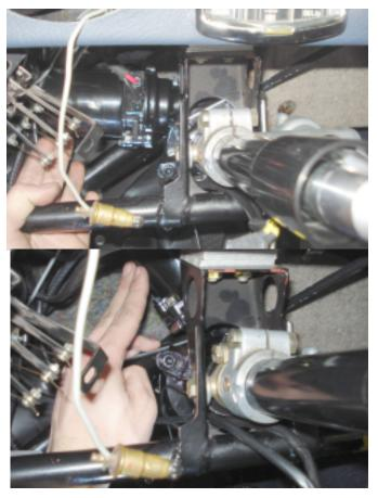
14.Install the electromotor on the EZ-unit and turn the unit in the right position. Subsequently fasten the mounting clamps.
