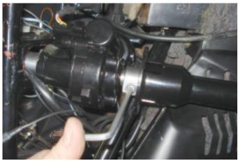
10. Fasten the output shaft to the EZ unit and tighten the retaining bolt securely. Do not forget, to fit the universal joint in the engine compartment.
