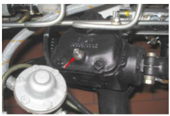
4. Put the steering wheel in centre position. Demount the plug from the wheelhouse. The wheelhouse can be fixed in the centre position with an original Mercedes pointed bolt (m10x1 conical). If this is not present, then mark the position on the steering shaft relative to the steering box.
