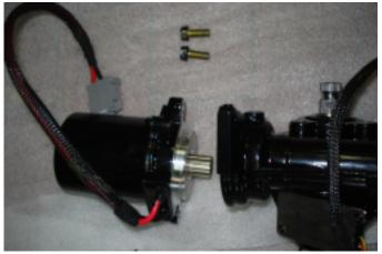
8. Remove the electric motor of the EZ unit.
