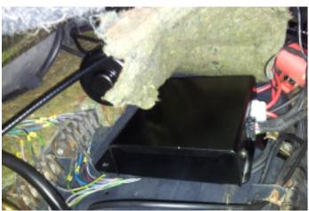
12. Place the ECU. Attach the base plate to the bolt from the air filter and to the bolt which retains the wiring.
