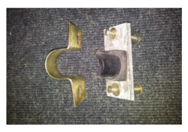
26. Put the omega shaped clamp back on the input tube and under the dashboard. Do not fasten the clamp yet. Do not forget to place the rubber back.
