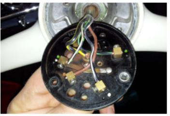
30. Use a Multimeter to determine the positions of the wires of the horn, indicator power, Left and Right.
