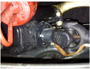
2. Put the steering wheel in a straight ahead position. Mark this position on the steering box and the steering shaft (see picture). If available, the steering box can also be blocked with an original pointed bolt to lock the steering in the middle position..
