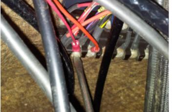
15. Connect the thin red wire (15+) to an ignition switched 12v plus (see point 2).
