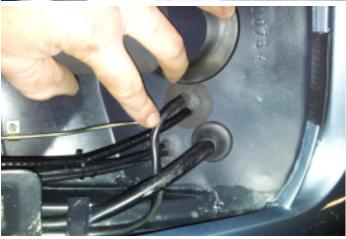
7. Pull the steering tube out of the universal joint by means of the steering wheel. Pull the wiring loom out of the steering tube and steering box and re-route it through the firewall to the area under the dashboard.
