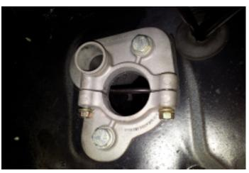
9. Loosen the clamps on the steering tube clamp on the firewall.
