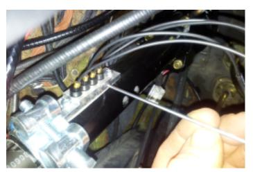
29. Mount the springloaded contacts in the aluminum holder so they align with the copper rings. DO not overtighten the grubscrews, it must be possible to pull the wire and hear it snap back due to the spring.
