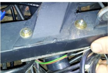
10. Remove the omega shaped bracket around the steering tube, under the dashboard. Please note, there is a rubber in between!
