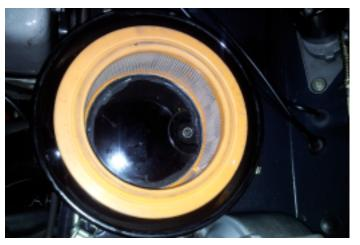
11. Open the top part of the air filter housing. Remove the bolt and replace it for a longer one (M6 x 25 mm).
