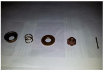
31. Mount the signal ring. Note the order of the connecting parts!
