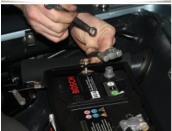
3. Find an ignition switched 12V plus wire and mark this. Subsequently, remove the earth cable from the battery.
