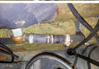
16. If necessary, loosen the banjo bolt from the brake booster to rotate the vacuum line from the brake booster. By doing this, you will create space for the assembly of the EZ steering column.
