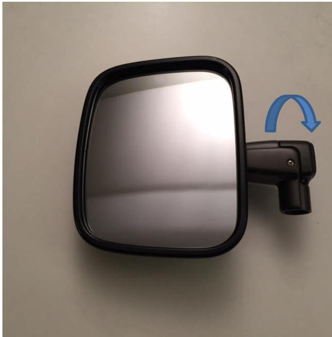
The mirror handle can be rotated by 180 degrees to fit on either the left or right side.
