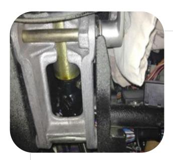
**Step 4.**Loosen the U-joint which is fitted behind the column.
