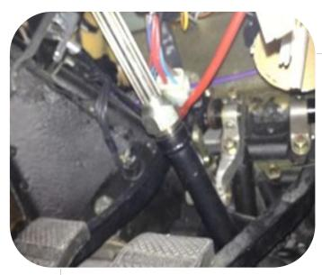
**Step 5.**Remove the steering shaft.
