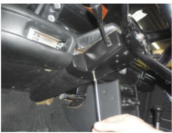
3. Remove the 4 retaining screws from the upper steering column cover.
