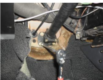
16. Remove the bolts from the original steering column at the firewall.
