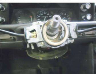
31. Check the position from the indicator reset and adjust it if necessary.
