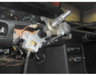
29. Install the steering column switches and horn contact ring to the column.
