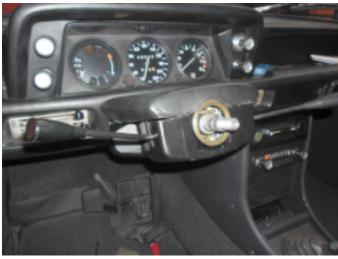
33. Install the remaining covers onto the steering column.
