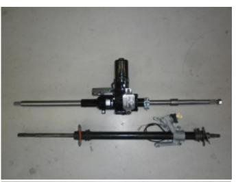
23. Put the original column next the EZ column and measure the length from the original shaft against the tube. Use this measurement to get the right measurement to cut the orignal steering tube.
