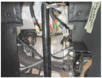
12. Disconnect the connectors from the steering column.
