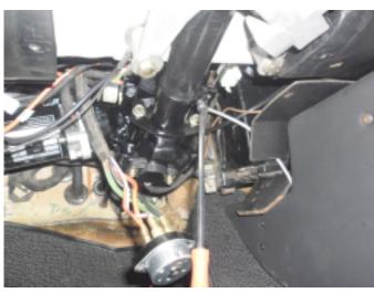
28. Once everything is installed correctly tighten the clamp bolt which holds the original pipe to the EZ unit.
