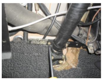
9. Remove the bracket which holds the steering column cover.
