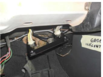
20. The connectors now can be installed inside the EZ mounting plate. Which can be installed at the original location.
