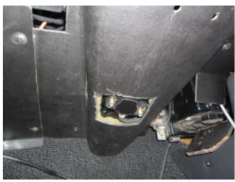
32. In some cases it can be necessary to cut a piece from the lower cover to give room to the EZ unit. If needed, use the EZ unit to determine where to cut.
