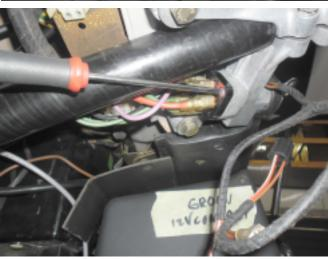
14. Remove the connector from the rear off the ignition lock.
