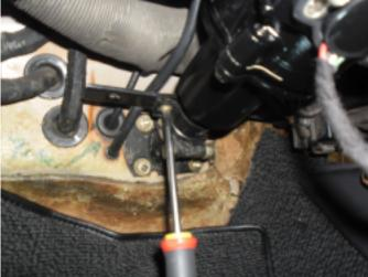
30. Install the lower bracket to the column.
