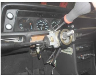
13. Remove the steering columnswitches and horn contact ring.
