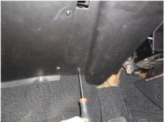
7. Now remove the lower parts from the cover over the steering column, this is fitted with some screws.
