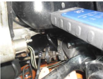
15. Remove the steeringshaft from the steering box. This is fitted with a clamping bolt. You can reach this bolt from underneath the car.
