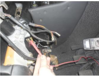
10. Find an ignition switched plus and mark this wire. the battery earth can be disconnected now.
