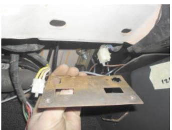
19. Remove the connectors from the upper mounting plate, the plate itself can be removed afterwards.
