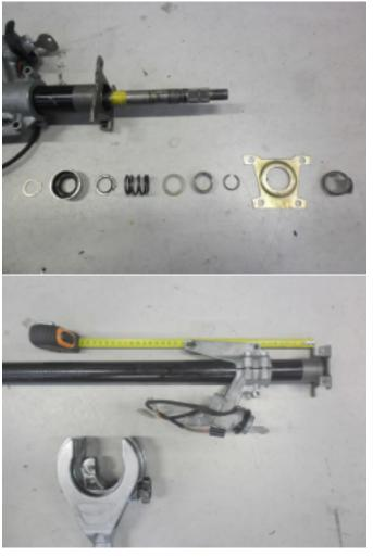
24. Remove all installation parts from the steering shaft so that it can be removed from the tube (watch the steering lock). Cut the pipe, use the measurements from point 23 to determine where to cut.
