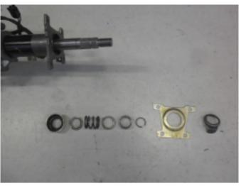
26. Now install all remaining installation parts back onto the EZ unit.
