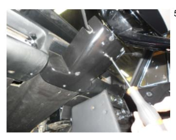
5. Remove the lower cover, this is fitted with 4 screws.
