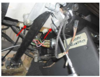
17. Now remove the upper 2 mounting bolts from the column.
