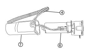
Slide rubber grommet on wire harness into slot of motor cover. Install motor cover onto motor.
