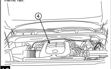
Route shorter leg of wire harness down driver side fender well and under vehicle outside of
