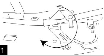
Slide motor assembly onto drive shaft and mounting bosses of driving linkage assembly. Use socket head cap screws (9) and tighten to 8 ft-lbs / 11Nm.
