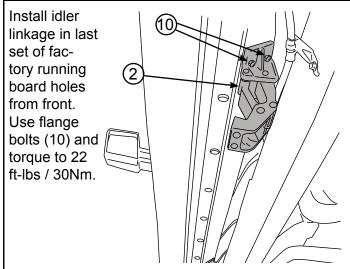
Repeat linkage installation on passenger side.
