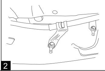
Install motor linkage on driver side in second set of factory running board holes from front. Use flange bolts (10) and torque to 22 ft-lbs / 30Nm.
