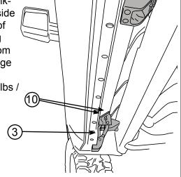
Install running board. See step 7 for alignment.
