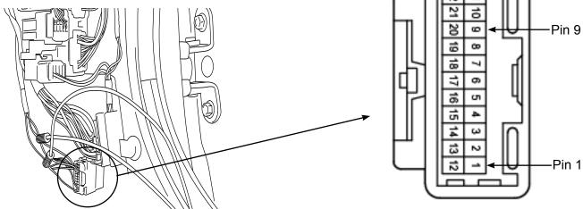
Insert plug from wire harness onto motor.
