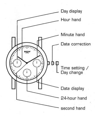
The 24-hour hand moves correspondingly with the hour hand and cannot be adjusted separately.
