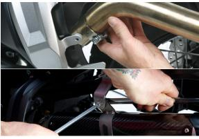
Make sure muffler is properly aligned, then tighten all the bolts in this order: Muffler mount bolt, muffler clamp bolt, slip-tube barrel clamp.
