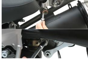
Install TBR muffler bracket with OEM mount bolt and nut, leave loose for now.
