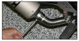
7. Before you run the bike, clean off all fingerprints and dirt, as any oily residue will etch the metal and become somewhat permanent when the system gets hot. Run the bike and enjoy. It is normal for some white smoke to appear the first time you start the bike. This is packing/manufacturing oil from inside the pipe burning off. Check for gaps or leaks. If you find a leak, a little high temperature silicon sealant should fix it. After 50 to 100 miles, recheck all fasteners for tightness.
