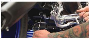
Apply small amount of anti-seize to O2 sensor threads and install O2 sensor into head pipe.
