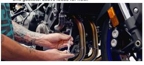
Attach supplied muffler mounting bracket using two 8x30mm bolts and two 8mm flange nuts.
