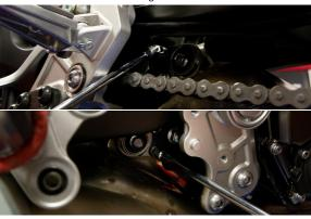
6. Remove OEM exhaust assembly.
