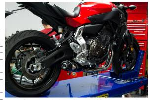
17. Before you run the bike, clean off all fingerprints and dirt, as any oily residue will etch the metal and become somewhat permanent when the system gets hot. Run the bike and enjoy. It is normal for some white smoke to appear the first time you start the bike. This is packing/manufacturing oil from inside the pipe burning off. Check for gaps or leaks. If you find a leak, a little high temperature silicon sealant should fix it. After 50 to 100 miles, recheck all fasteners for tightness.
