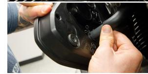
Remove OEM gaskets from back of air box to be used with TBR Comp-V.
