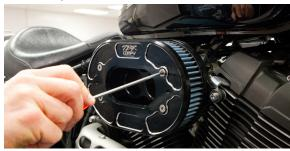
8. Install plug cap on V-Stack and tighten two mounting bolts to
