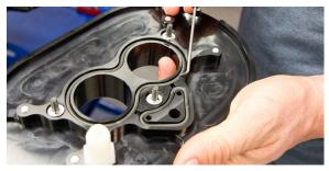
Remove rubber grommet and spacer and install on Comp-V backing plate.
