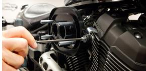
Install TBR air filter and face plate. Tighten the four socket head cap screws.
