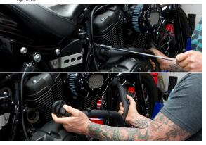
Slide TBR flanges over head tube and loosely install headers using OEM hardware and gaskets.
