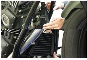
Loosely Install supplied TBR heat shield to rear header and install TBR rear header using OEM hardware and re install 02 sensor.
