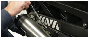
14. Tighten header flange bolts.
