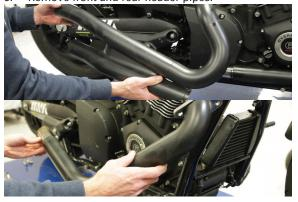
6. Loosely Install supplied TBR heat shield to front header.
