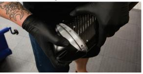
Remove all existing packing material from the perforated core, if your canister came with a stainless steel wool wrap around the core leave this in place.
