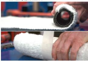
Insert the newly wrapped perforated core into muffler sleeve. Replace o-ring on outlet flange and then install into the sleeve. Make sure the perforated core seats fully into both inlet and outlet flange completely.
