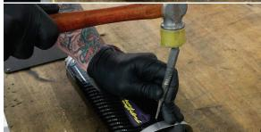
Separate the outlet flange and inner core from the muffler sleeve.
